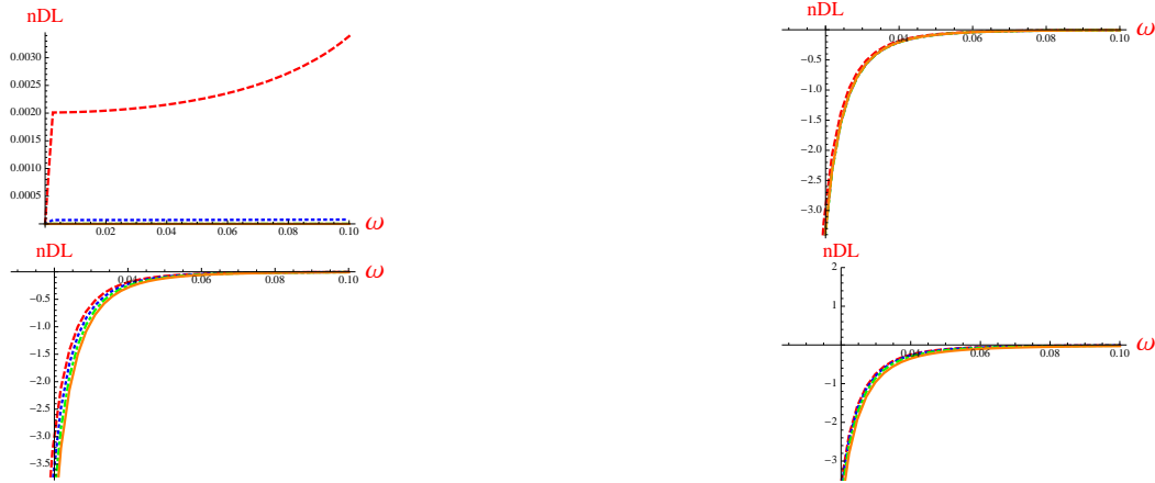
Figure 6: Zoom of the index n_{DL} in the region of significant negative refraction (low \omega ) for \kappa^2 = 10^{-10}, .1, .2, .3 and for \kappa^2 = 10^{-10}, .1, .2, .3 and for T/T_c = .9 (red) .75 (blue) .6 (green) and .45 (orange).
