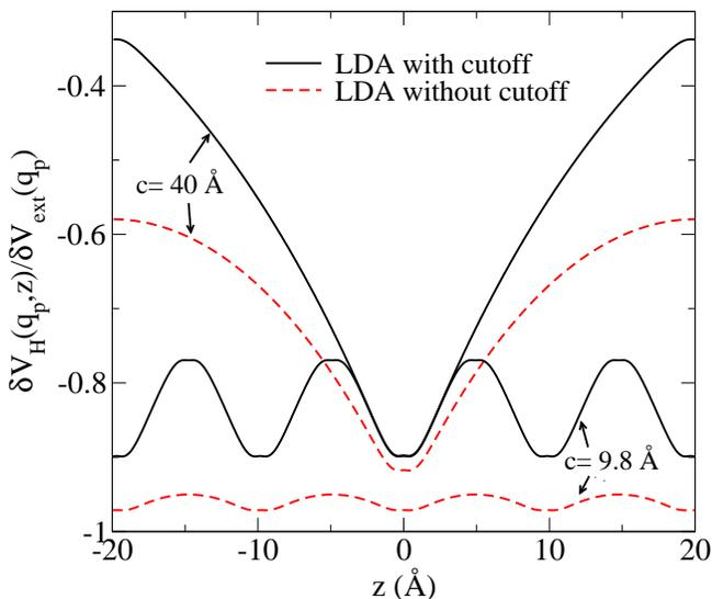
FIG. 3. (Color online) The Hartree potentials are plotted in the out-of-plane direction with and without cutoff and for two different interlayer distances  $c \approx 40 \text{ \AA}$  and  $c \approx 9.8 \text{ \AA}$ . The calculations were performed for doped graphene with  $\varepsilon_F = 0.25 \text{ eV}$ , at  $|\mathbf{q}_p| \approx 0.32 |\Gamma - \mathbf{K}| \approx 1.2 k_F$ .
