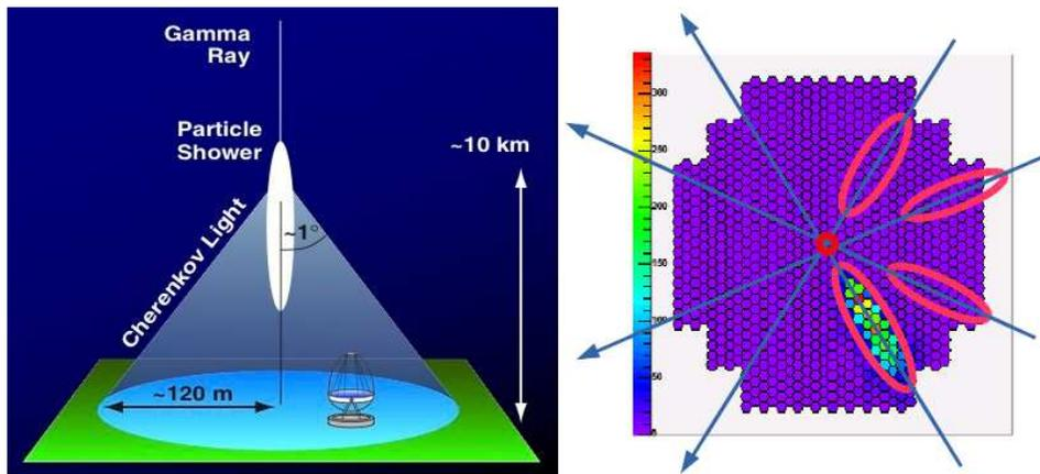
Figure 1. Detection of gamma-rays using Cherenkov telescopes. *Left*: schema of a particle shower entering the atmosphere. The Cherenkov light is caught by one or several telescopes. *Right*: image of the shower on the camera of a telescope and basic reconstruction of the event direction for four telescopes.
