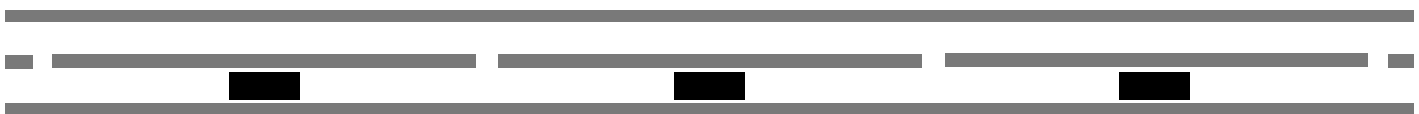
Figure 6. Chain of coplanar waveguide resonators (central and grounded conductors indicated by grey lines), that each couple to a transmon qubit (black boxes). Neighbouring resonators are coupled via a capacitance (indicated by the small gaps in the central conductor).
