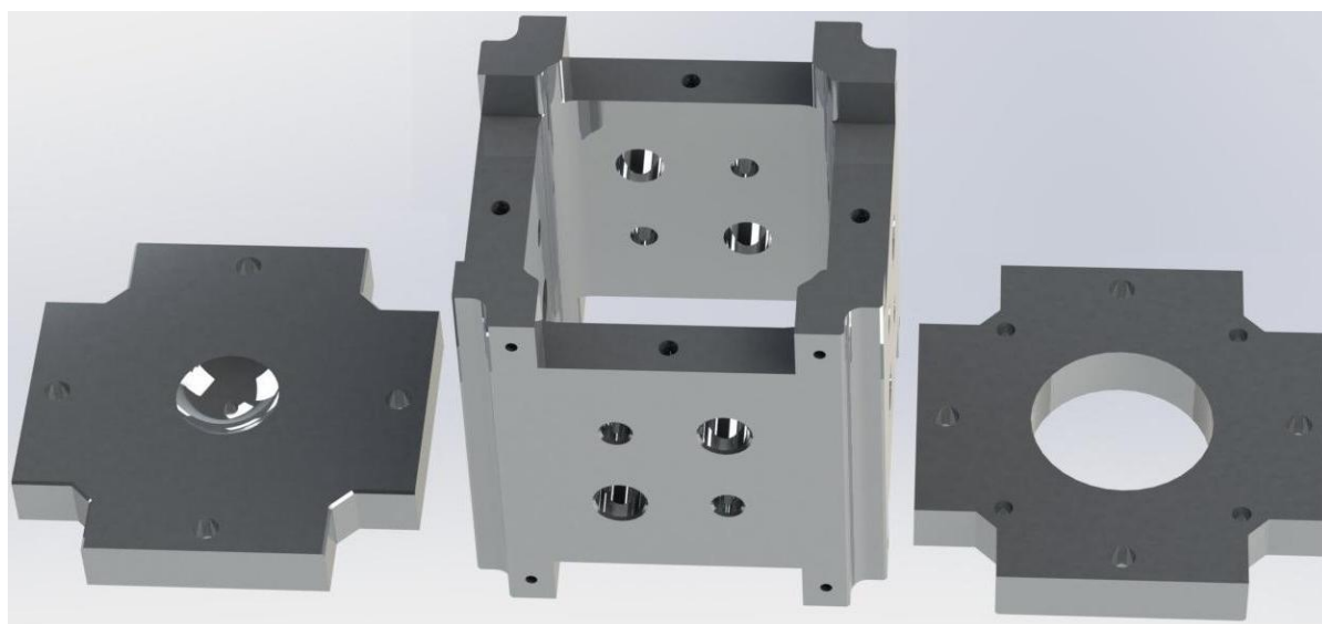
Figure 5: CAD model of the disassembled housing
