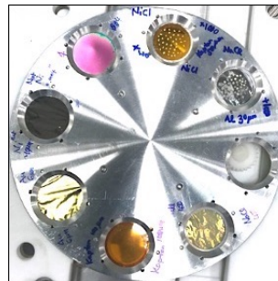
Figure 3: Picture of the 8 position aluminum target wheel used in the middle of LENZ.
