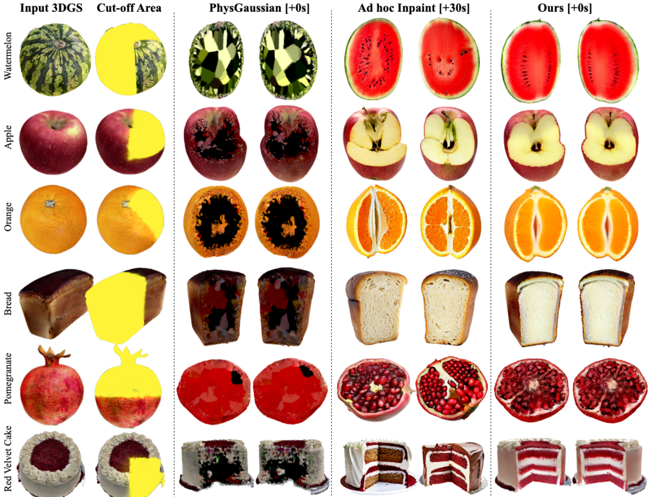
Figure 6. Qualitative comparison with PhysGaussian and 2D inpainting using stable-diffusion-2-depth[31] (which requires \sim 30 s for 70 DDIM sampling steps per view). 3DGS from FruitNinja shows better texture consistency and visual quality without any optimization.
