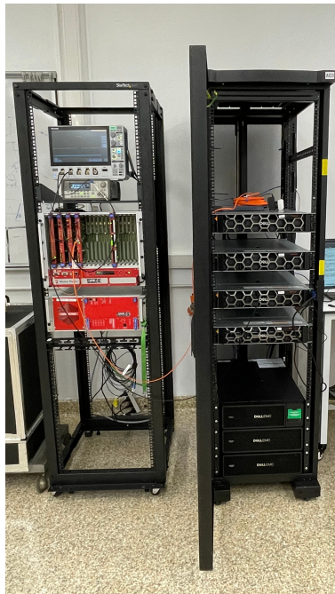
Figure 21. SABRE DAQ electronics (left) and server units (right).
