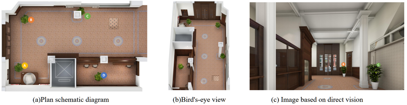
Fig. 1. When the camera is deployed at a position directly facing the gate and only direct vision is used, due to the irregular shape of the indoor space, the direct vision of the camera is blocked. Among the four plants placed in this space, only two can be observed, and two plants are invisible in the occluded area.
