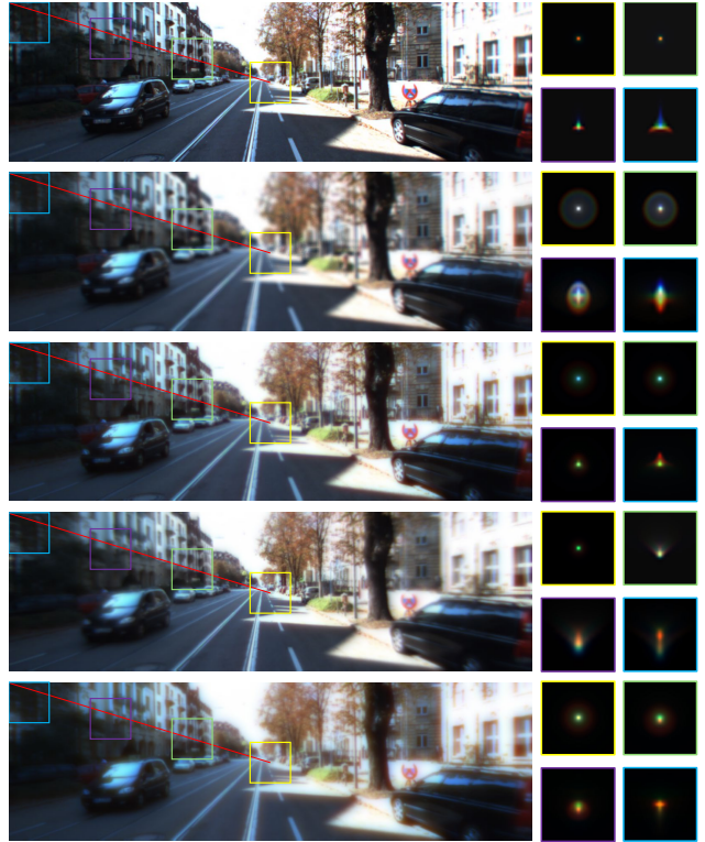
Figure 7. PSF illustration from severity 1 to 5. The PSFs of 4 different fields of view are shown.
