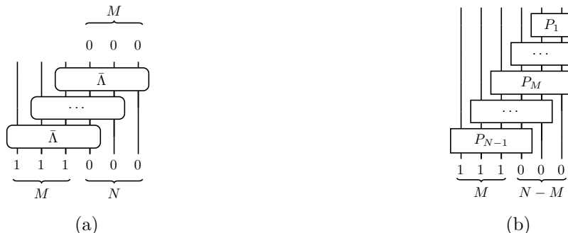
Figure 2: Realizations of Bethe states. Fig. 2a depicts the MPS of the CBA, whose \bar{\Lambda} is non-unitary (rounded corners). Fig. 2b depicts ABC, where P_k are unitaries (square corners).
