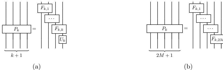
Figure 16: Factorization of P_k into two-qubit unitaries and single-qubit rotations at the free-fermion point. Fig. 16a depicts the factorization of short unitaries ( 1 \leq k < 2M ). Fig. 16b depicts the factorization of long unitaries ( 2M \leq k < N ).
